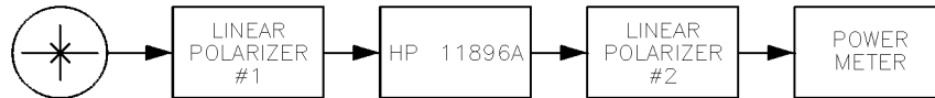
Figure B-1. Block diagram for testing the extinction ratio of the Agilent 11896A.
